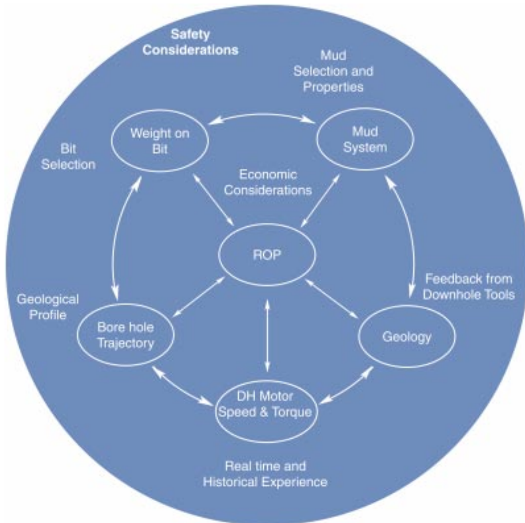
Figure 5 – Example of Feedback Loops in the Drilling Process
